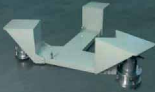
D. Platform for minimum working height and very low center of gravity
