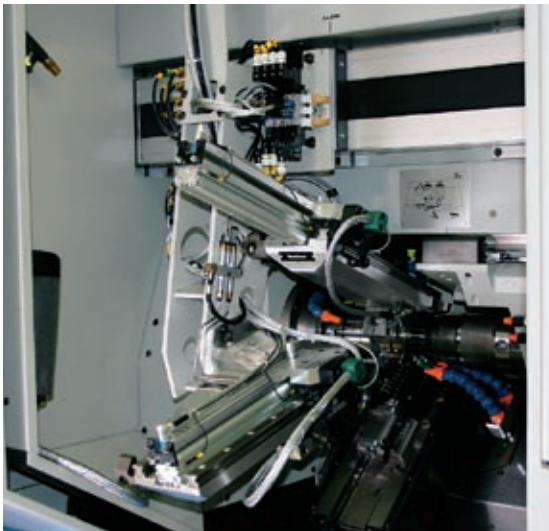
Work area with grippers in load / unload position
