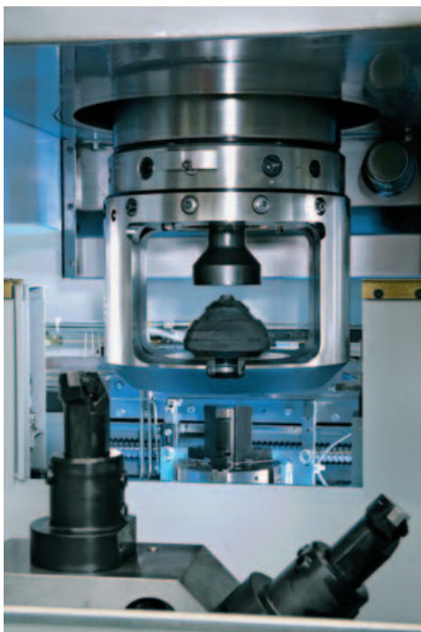
▼ Internal machining of the bearing journals on a VSC 400 (machine shown in pick-up position)
