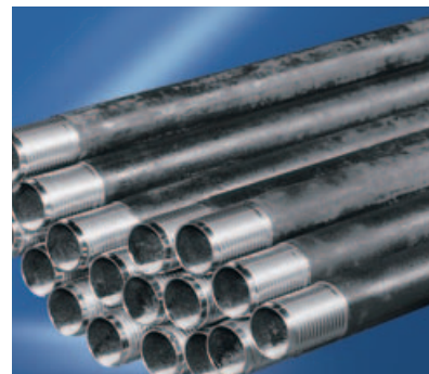
▶ Casings with external thread machined on USC 21
