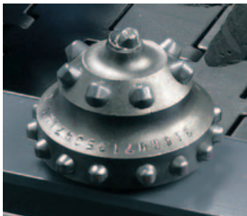
◀ Carbide tipped rock bit cone
