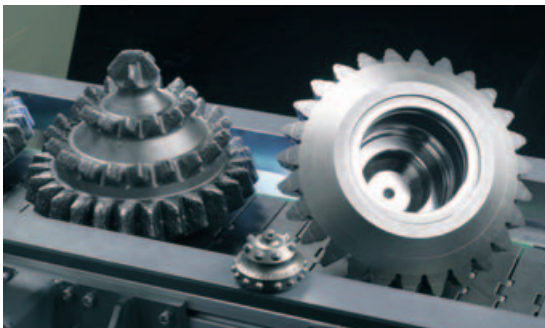
▲ An external view of rock bit cones and a view of the finish-machined internal bearing journal
