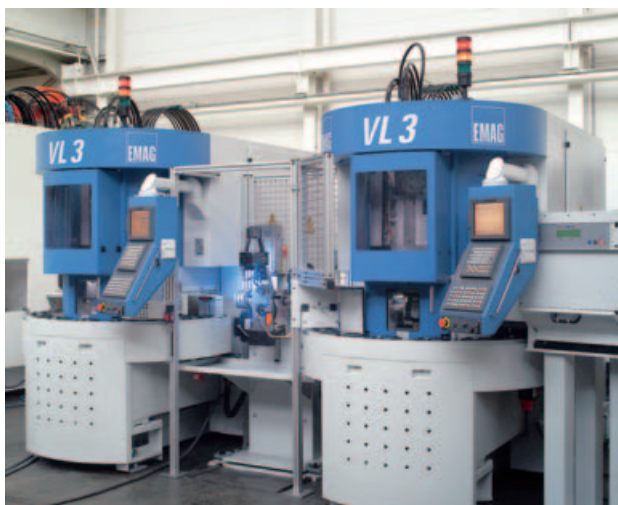
◀ 2 machines of the VL 3 series, connected by a transfer station
