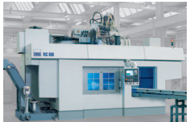
▲ VLC 800, used to machine the larger coupling sleeves
