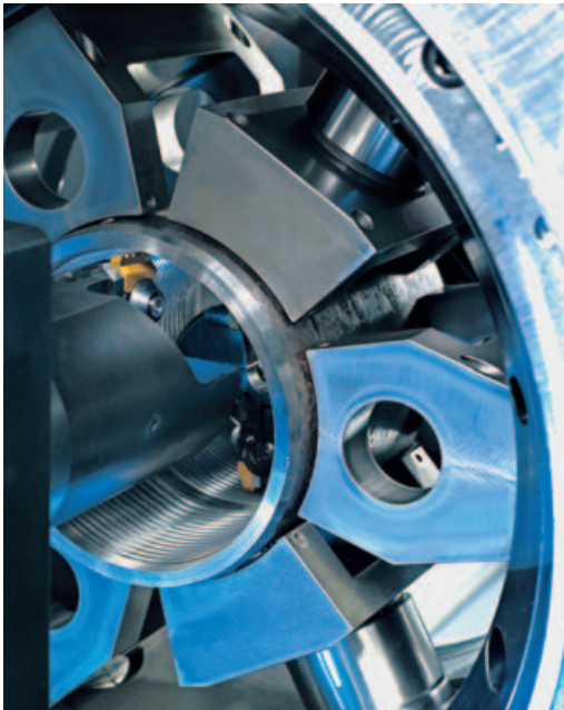
▲ Machining of coupling sleeves – both ends simultaneously – on a USC 27
