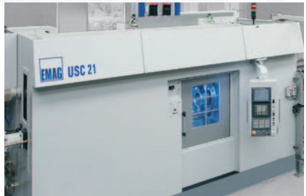
▲ USC 21 for the machining of vehicular hydraulics components
