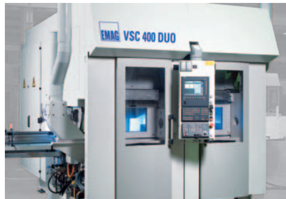
▲ VSC 400 DUO for the simultaneous execution of OP 10 and OP 20
