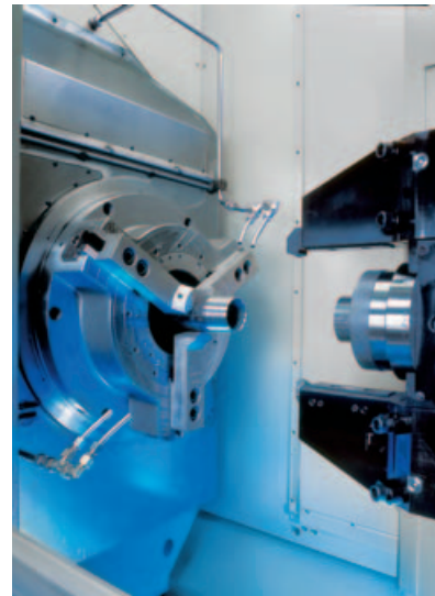
▶ API thread on an ascending tube, machined on a USC 11
