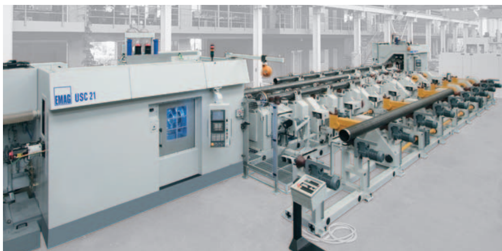
◀ USC21 with machine- specific tube handling system
