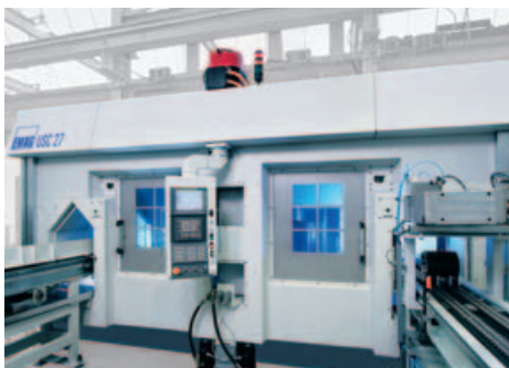
▼ USC 27, for the machining of coupling sleeves
