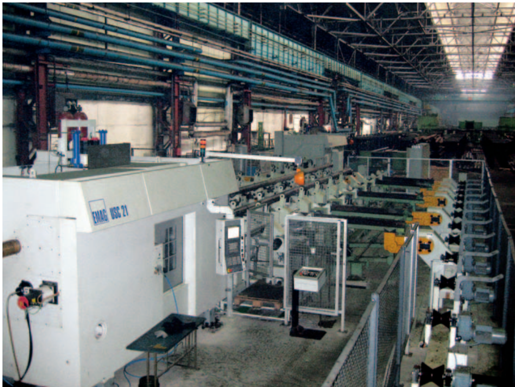
Complete-machining of tubes
