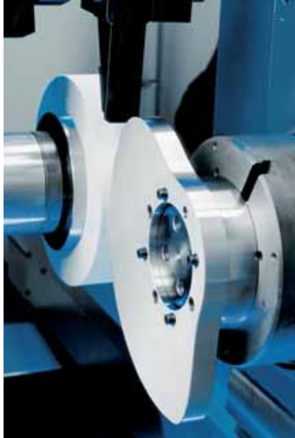
SK 204 machining area Grinding a radial cam
