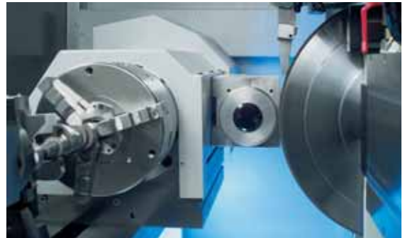
Dressing a ceramic bonded CBN grinding wheel with a live diamond wheel
