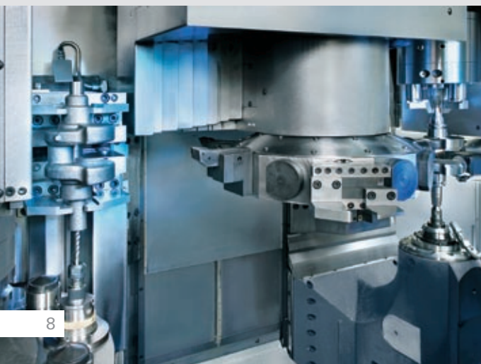
OP 10 + 20 Cutting to length, centring, turning (VTC 250 DUO)
