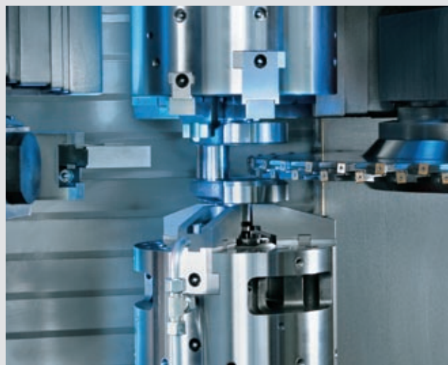
OP 30 milling the pin bearing (VTC 250 F)
