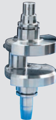
OP 30 milling the pin bearing (VTC 250 F)
