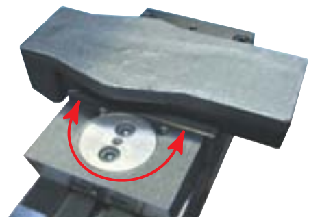
Jaws with 4 corrugated compensating supports; compensation \pm 9^\circ , movable jaw floating, without hold-down for clamping forgings
