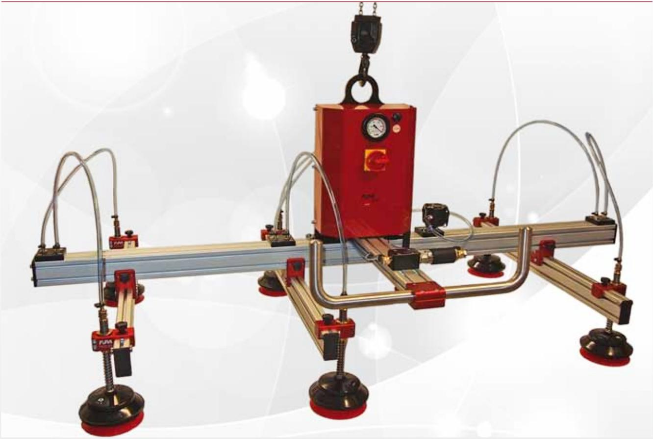
Vacuum lifters are superior to classic lifting devices with slings due to their faster and easier handling. Place the vacuum cup, press the manual slide valve and wait two to three seconds until the vacuum is generated. It is this easy to work with the vacuum lifter FIPA Spider!
