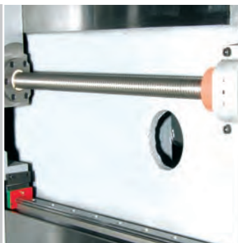
▲ Patented linear and box guideway structure (15300~15500)
