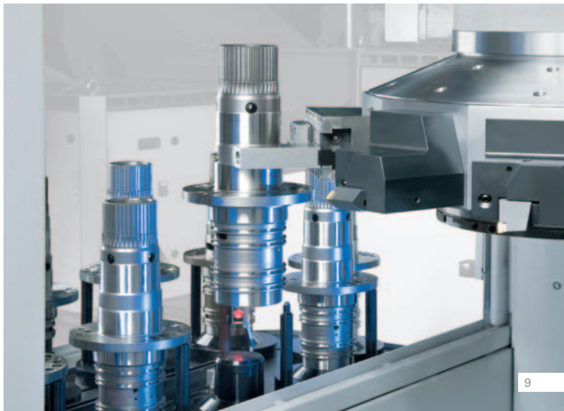
Integrated automation. A gripper in the turret enables the VTC 315 DS to load itself
