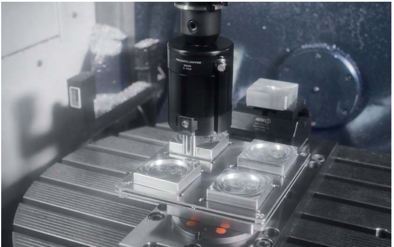
After processing, the finished workpieces are placed into the workpiece storage. This is clamped by means of the zero-point clamping system and can therefore be replaced quickly and individually.
