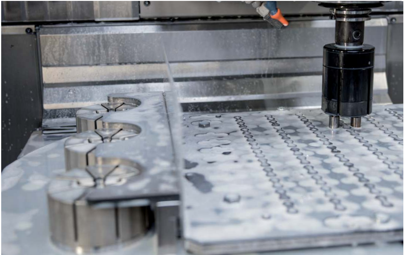
Unmanned shifts are now possible. The AMF gripper holds the workpieces between the workpiece storage and the three collets. Clamping system and storage are clamped by means of zero-point clamping system.
