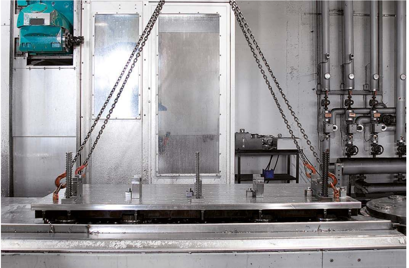
The cylindrical design of the pull-studs and the adapter in the clamping module guarantee a balance of height and length tolerances even at long distances.
