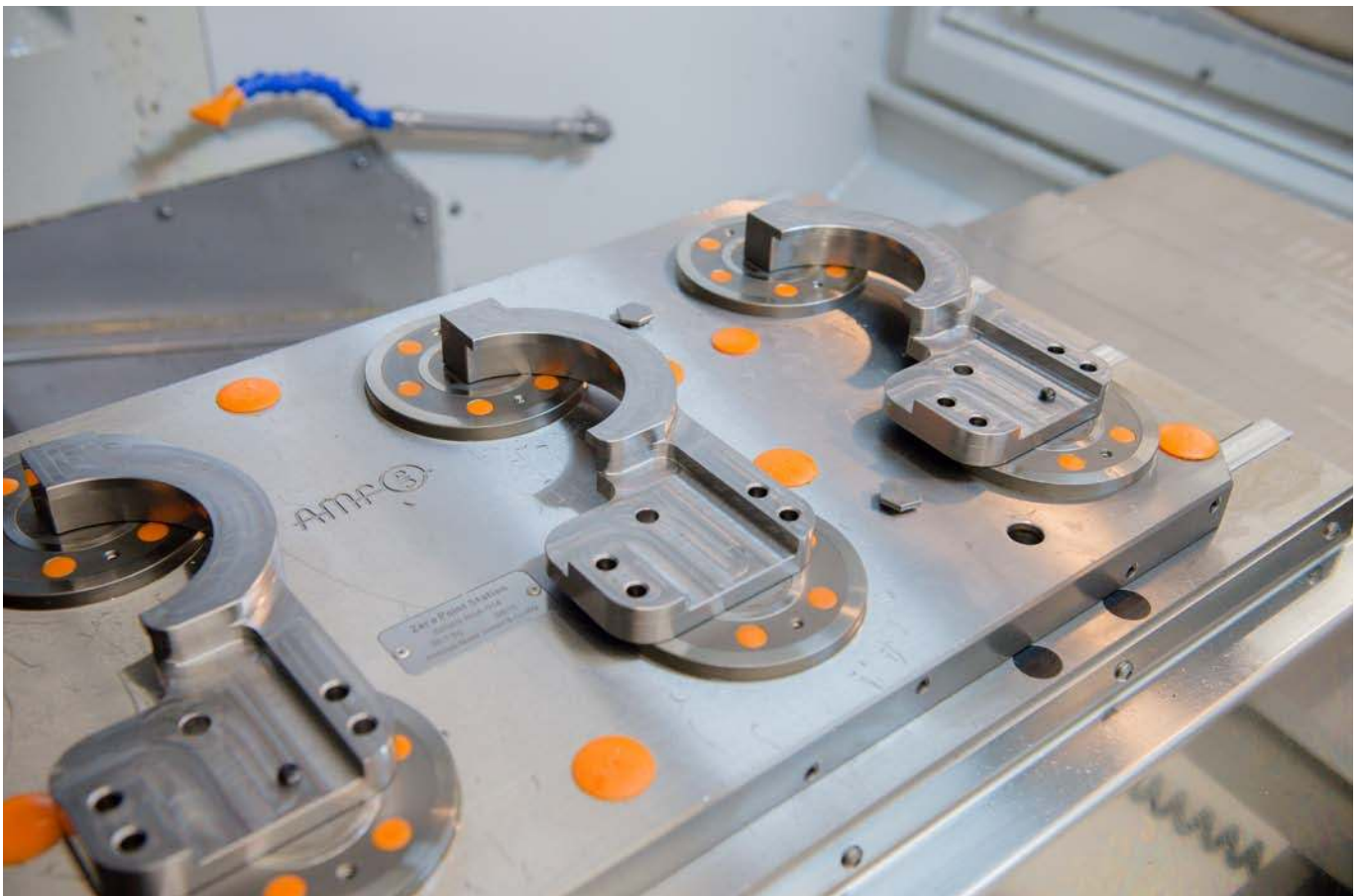
8-point clamping station for mounting different standard clamping equipment or direct clamping of the workpiece.
