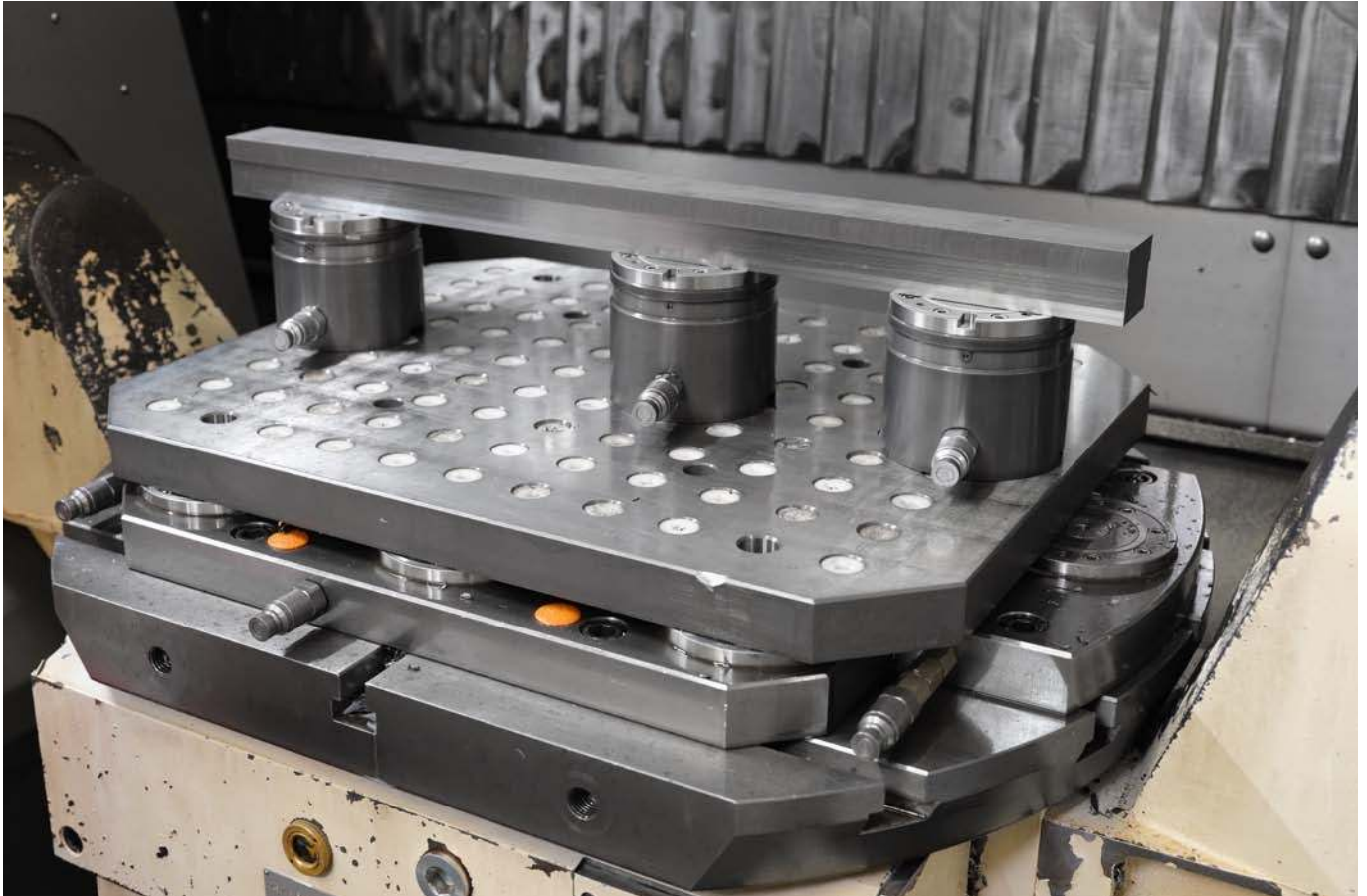
Ideal accessibility for 5-sided machining by our modular zero-point clamping technology.
