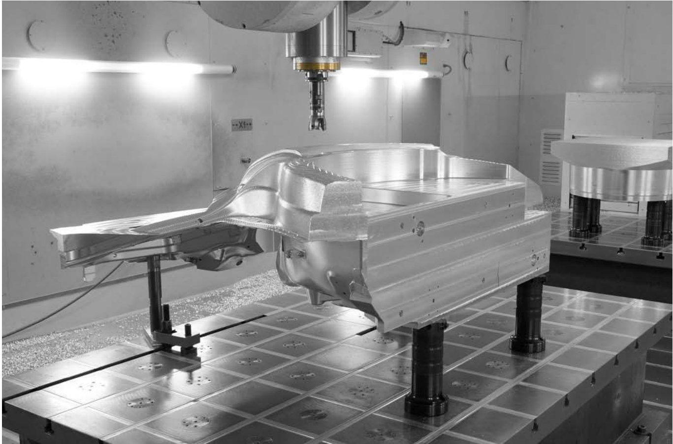
Direct clamping of the workpiece for large aluminium components. Zero-point clamping modules in the work table in conjunction with attachment and intermediate elements of the modular zero-point clamping system enable flexible clamping to be achieved.
