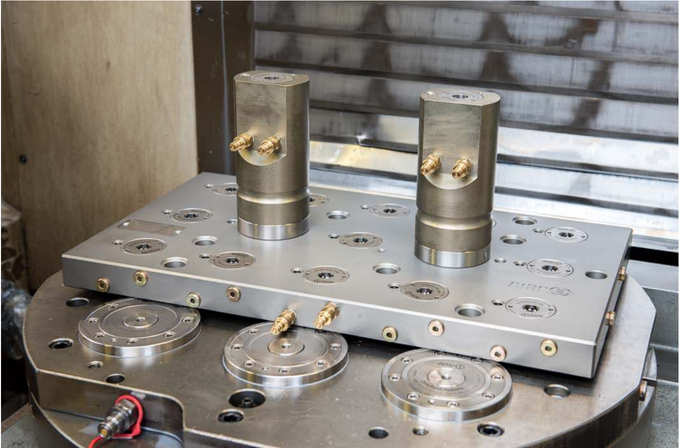
5-side machining by means of clamping brackets for direct clamping of the component.
