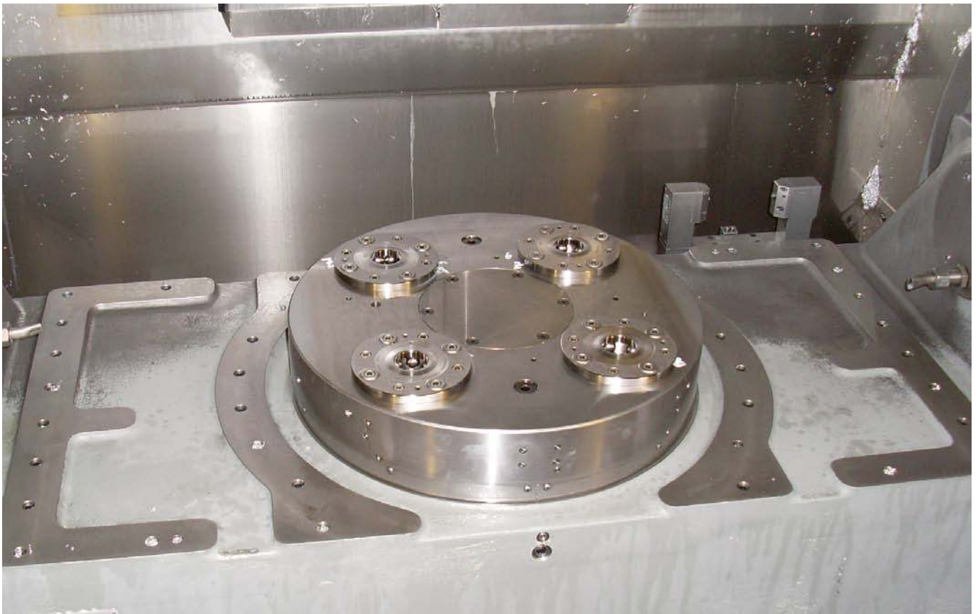
Automation solution with lock and support control as well as pull-stud sensor used in a fully automated production process with robotic loading.
