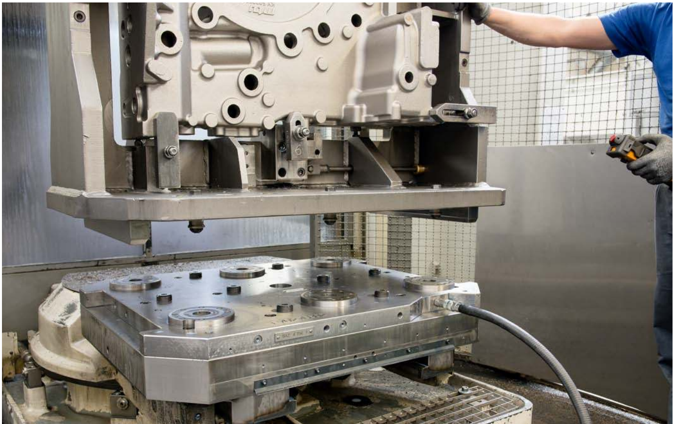
The two-section clamping pin system with a large intake catchment and the ball retainer-free module design makes it possible to change the clamping device ergonomically without tilting.
