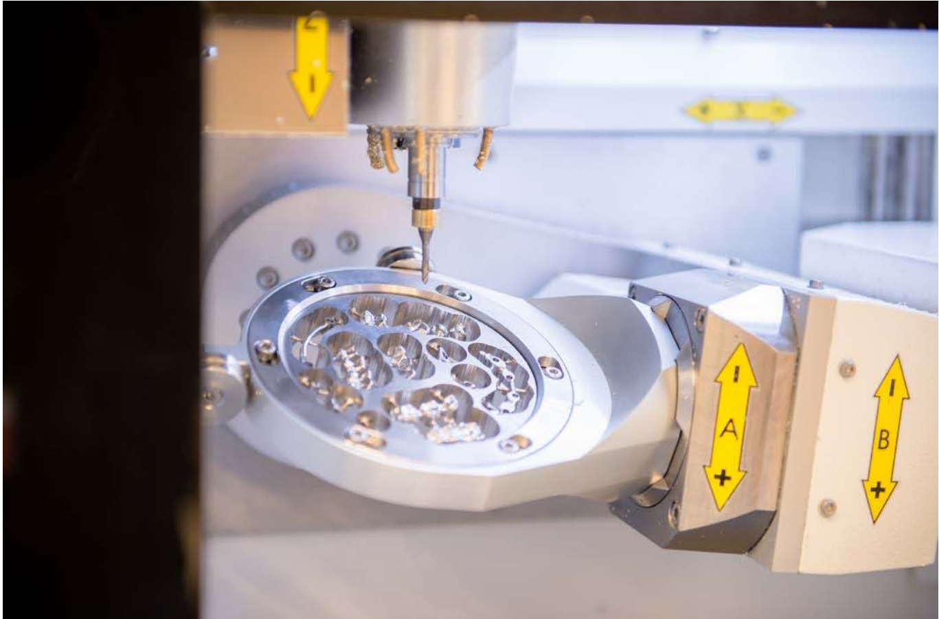
Fully automatic loading and clamping of circular blanks during the production of dental implants.
