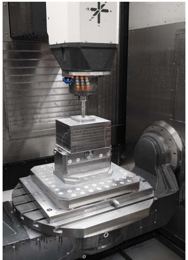
Ideal accessibility for 5-sided machining by our modular zero-point clamping technology.
