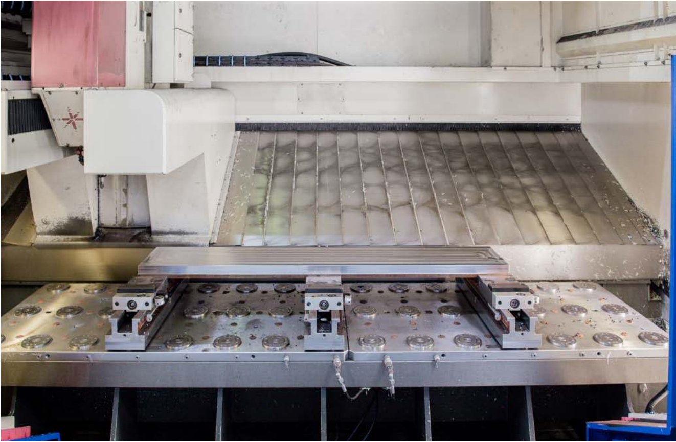
Easy alignment of multiple vices when machining long workpieces.
