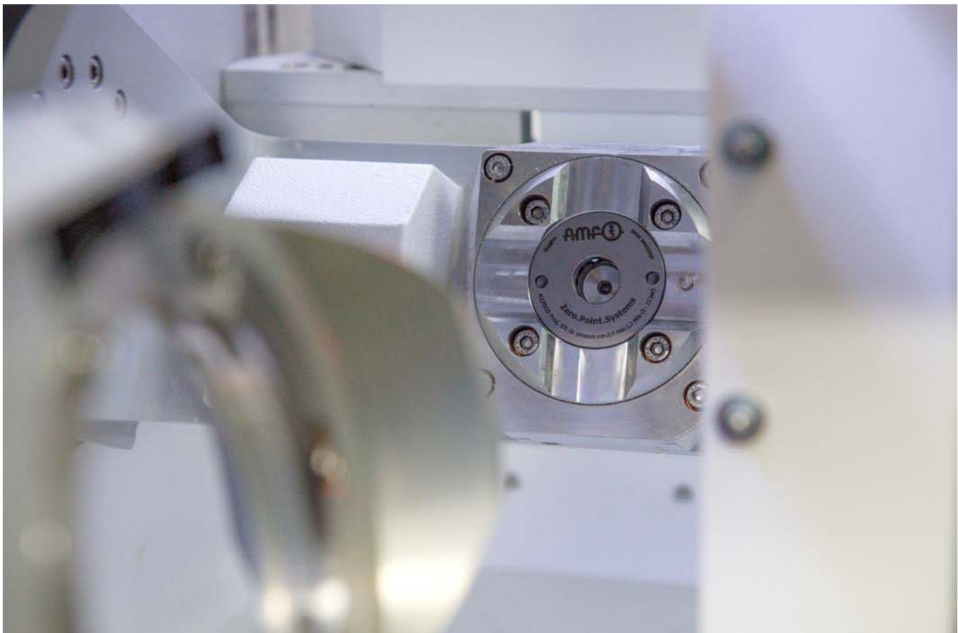
Fully automatic loading and clamping of circular blanks during the production of dental implants.
