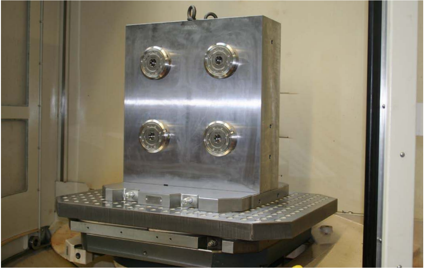
Integration clamping module as flange version for installation on clamping profiles.
