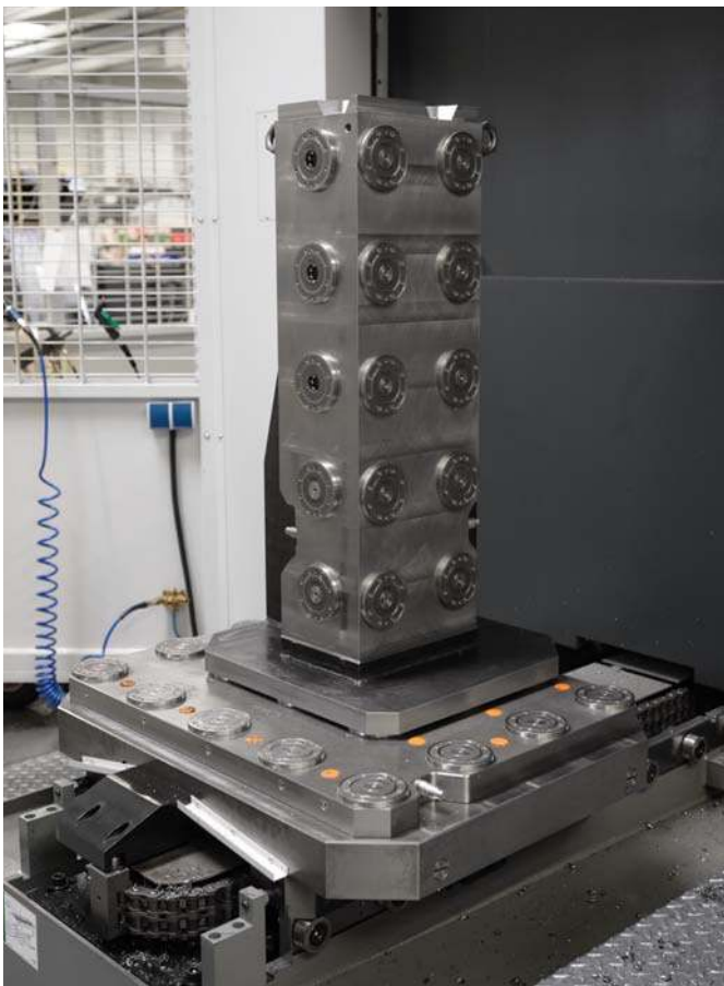
Ideal accessibility for 5-sided machining by our modular zero-point clamping technology.
