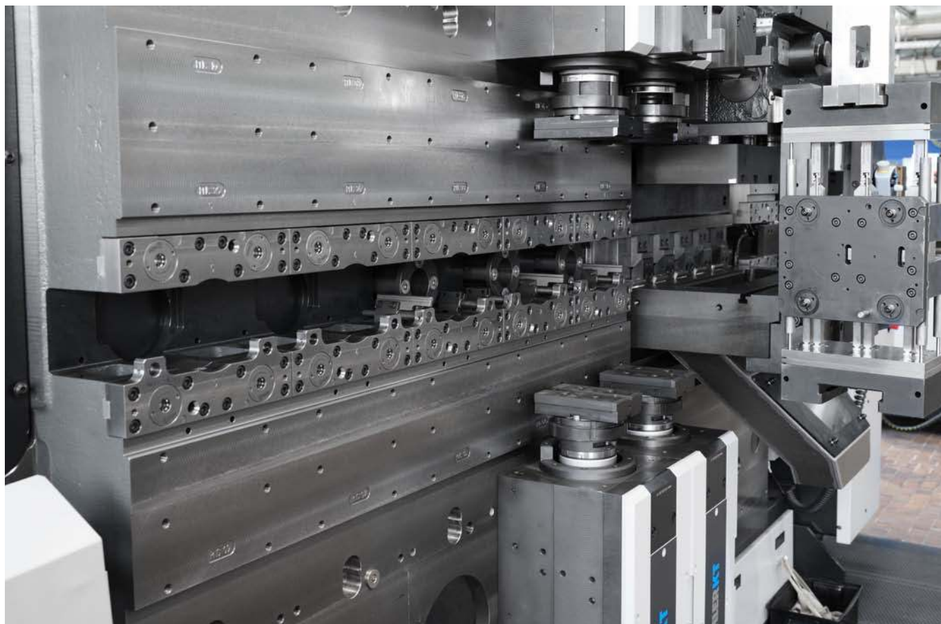
Each receptacle is equipped with four zero-point clamping modules. Thanks to the compact design, the clamping modules can be screwed in easily and flush.
