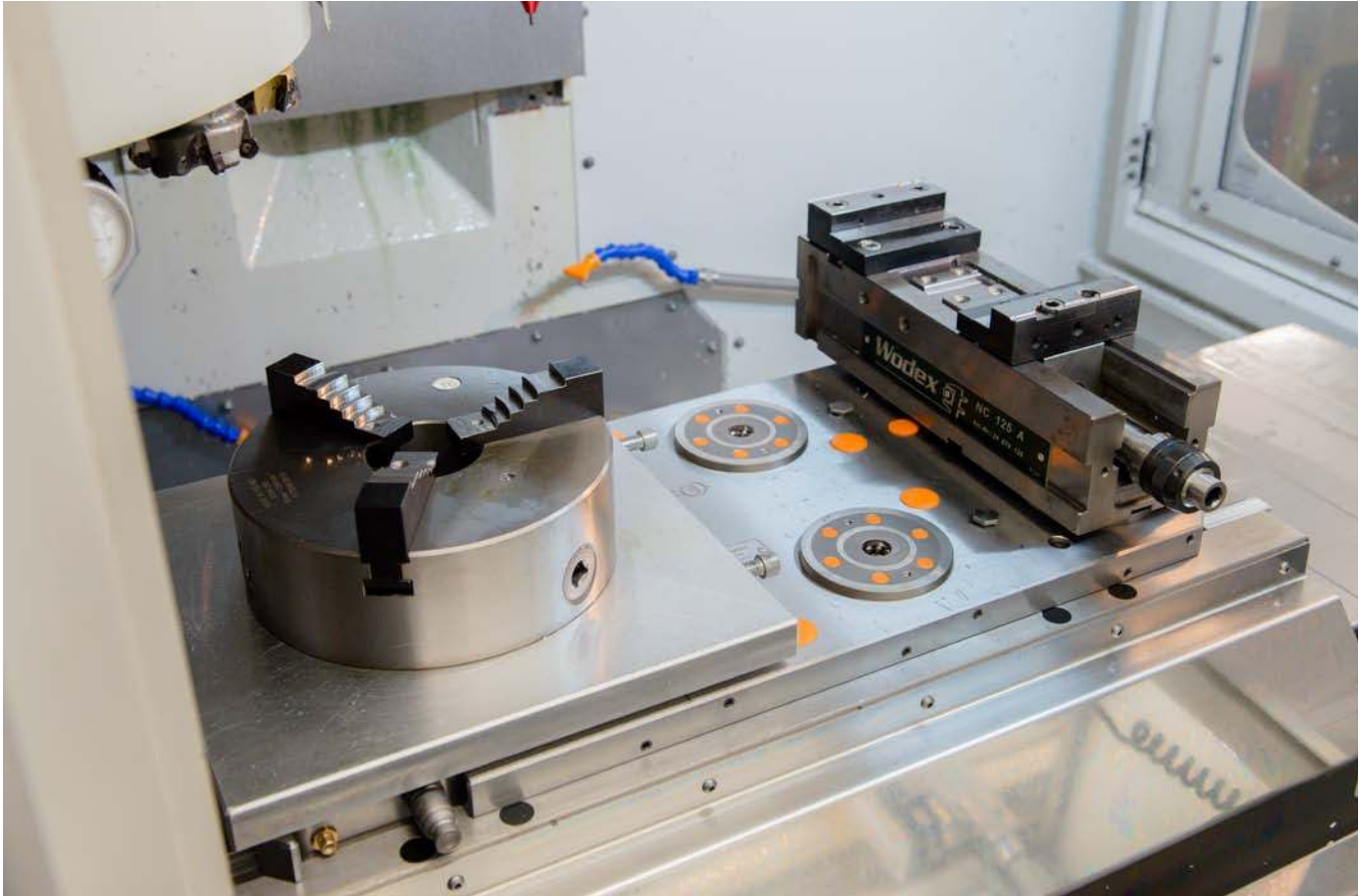
8-point clamping station for mounting different standard clamping equipment or direct clamping of the workpiece.
