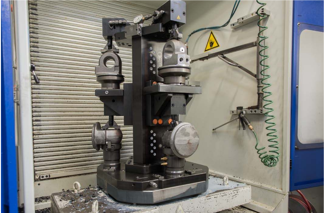
This complete clamping solution combines multiple clamp types in one clamping fixture. (modular clamping system, hydraulic clamping system as well as zero-point clamping technology).
