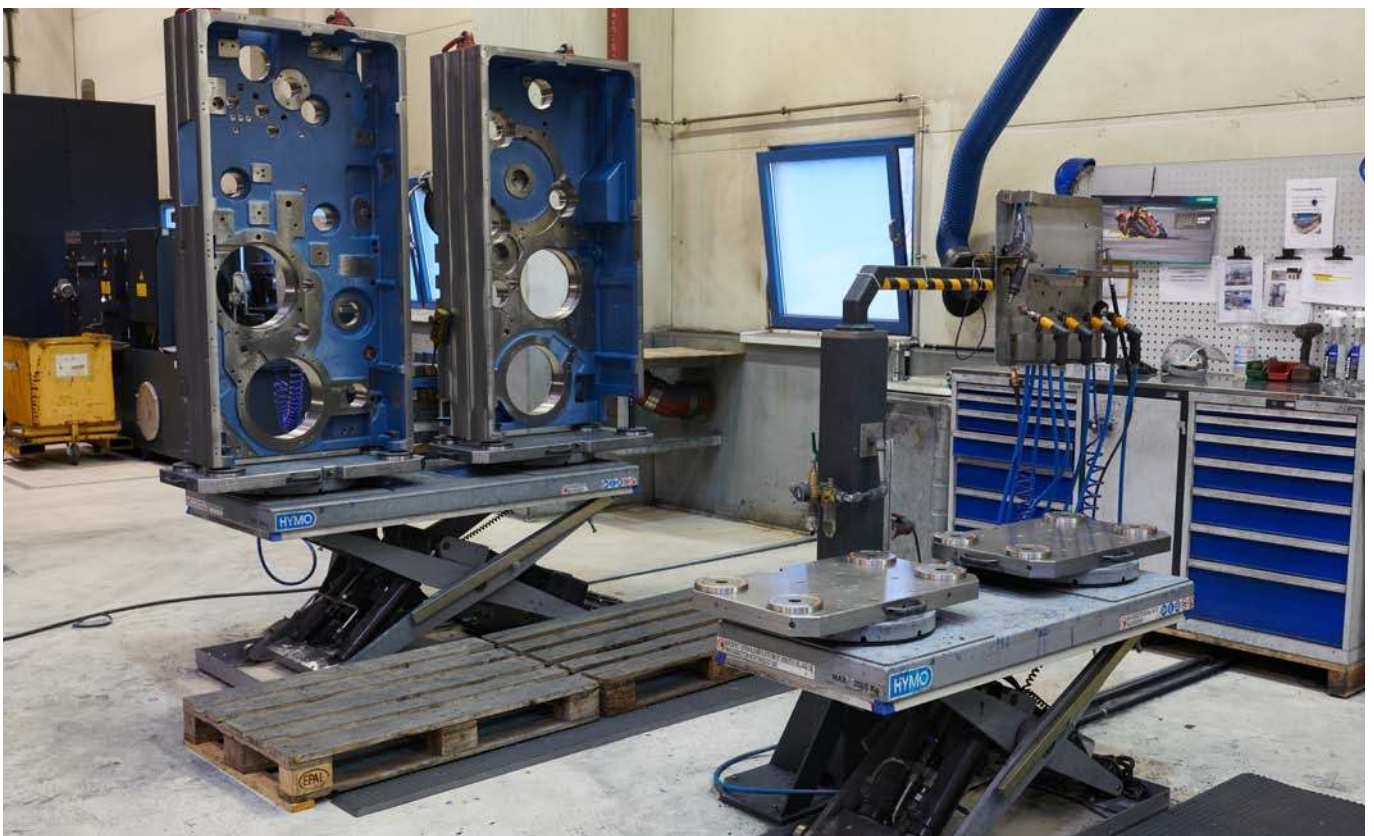
Lifting tables equipped with zero-point clamping technology for deburring the workpieces. As a result, the complete manufacturing process has been seamlessly optimised with the AMF Zero-Point-System.
