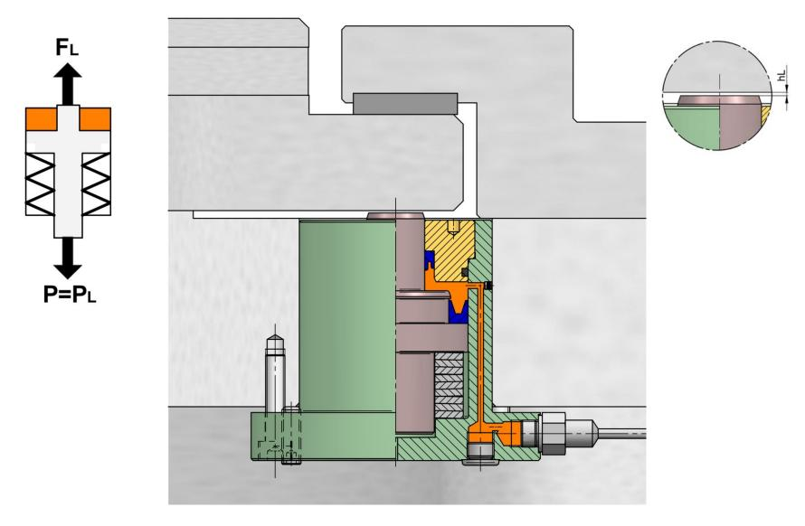
Release operation: with release pressure PL – disk spring package is getting stronger compressed – resultant release stroke hL of piston (ZDF-u 6.300: PL=max 230 bar / hL=1mm)
