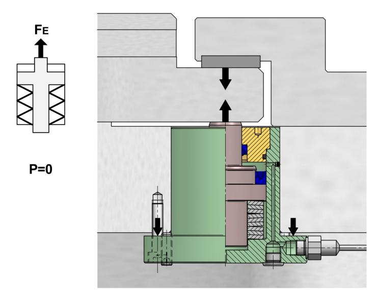
Clamping operation: release hydraulic pressure - P=0 bar disk spring package is clamping with nominal clamping force FE (ZDF-u 6.300: FE = 63 kN)
