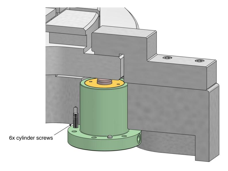
2 Mounting of spring clamping cylinder and fastening with 6 cylinder screws
