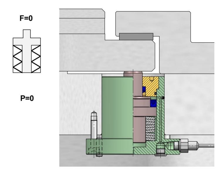
4 Initial position – without hydraulic pressure and without spring pre-load
