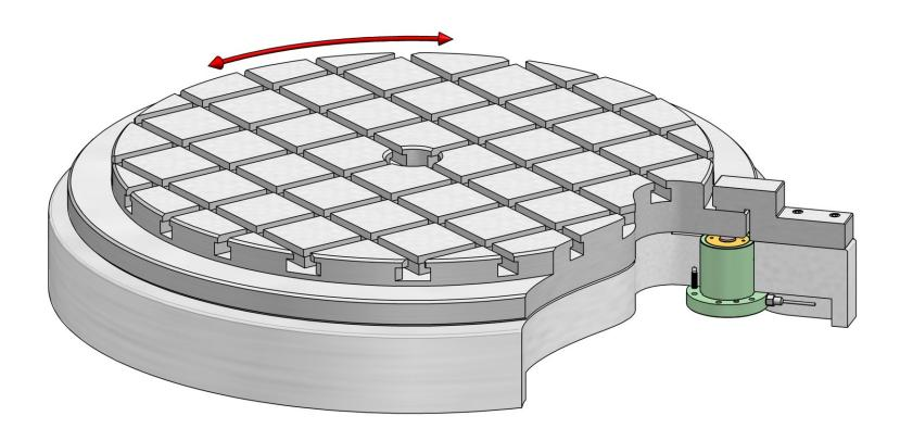
Release position: The clamping piston is loaded with release pressure PL, now the table can be turned to the new clamping position and can be clamped (P=0 bar) again
