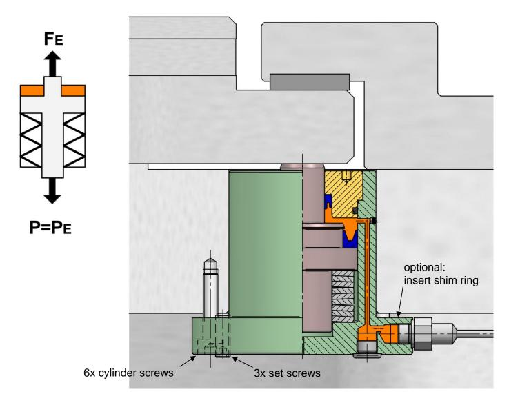
$6 \\ \text{Adjusting of spring clamping cylinder at setting pressure PE : Screw in cylinder screws till contact of the piston – exact positioning through setscrews or shim ring } \\$
