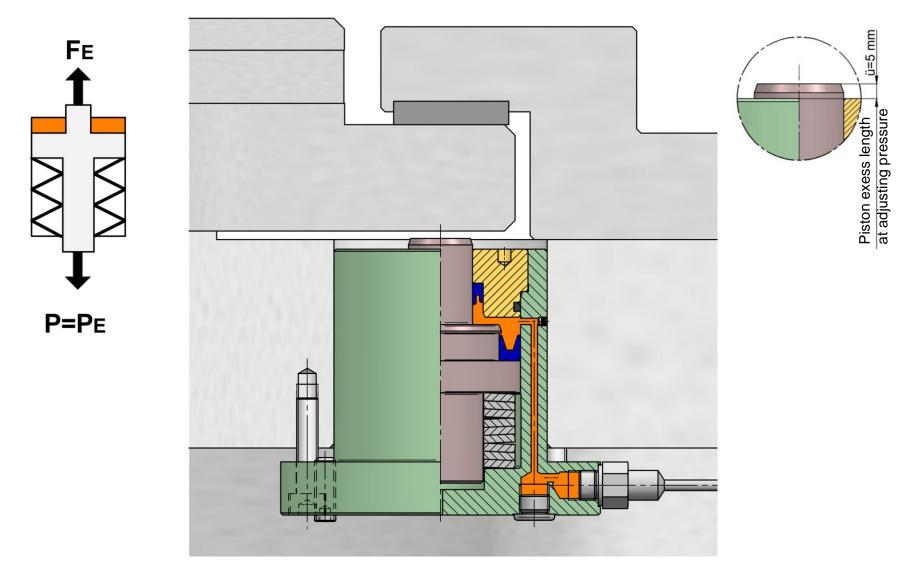
Load cylinder with adjusting pressure (size ZDF-u 6.300: PE=180 bar) – disk spring package is getting compressed – piston moves some millimeter backwards till ü = approx. 5mm
