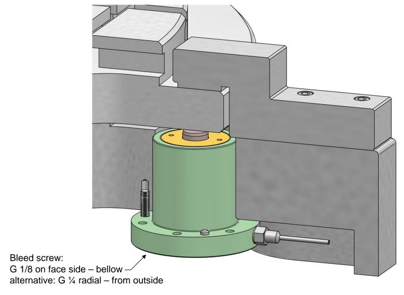
(3) Installation of hydraulic connection and bleed cylinder afterwards
