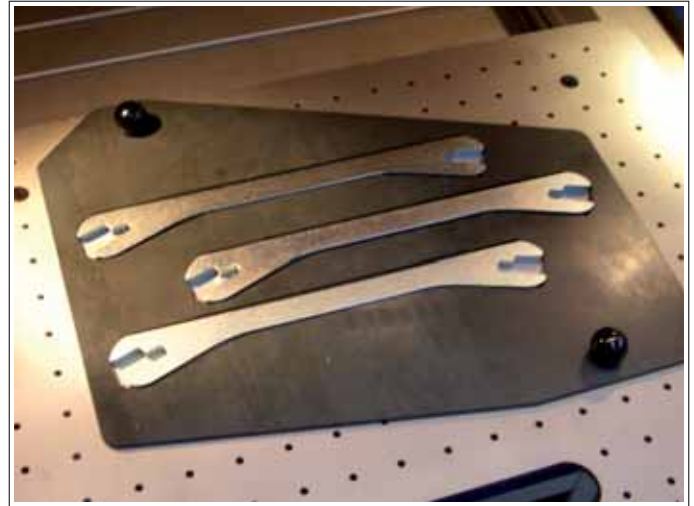
Precise marking of special wrenches is ensured by positioning with contour templates.
