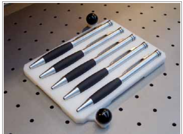
Ballpoint pens or other promotional gifts with complicated external shapes can be positioned precisely using contour templates.
