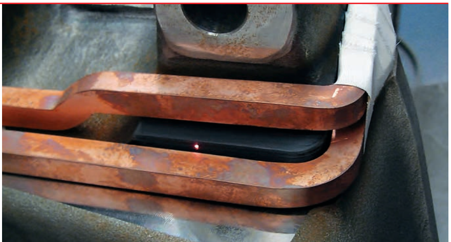
Component with adjusted inductor and pyrometer measurement spot to control the temperature
