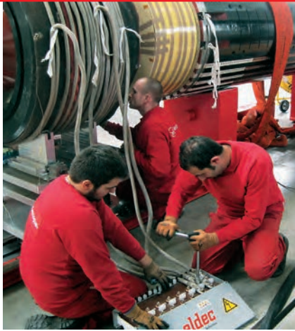
Winding and connecting the heating cables
