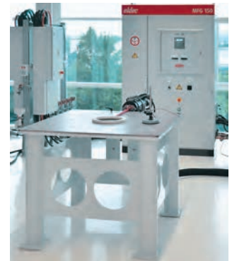
Solution – eldec MFG 150 generator with brazing bench
