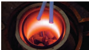
Molten copper in a carbon crucible
