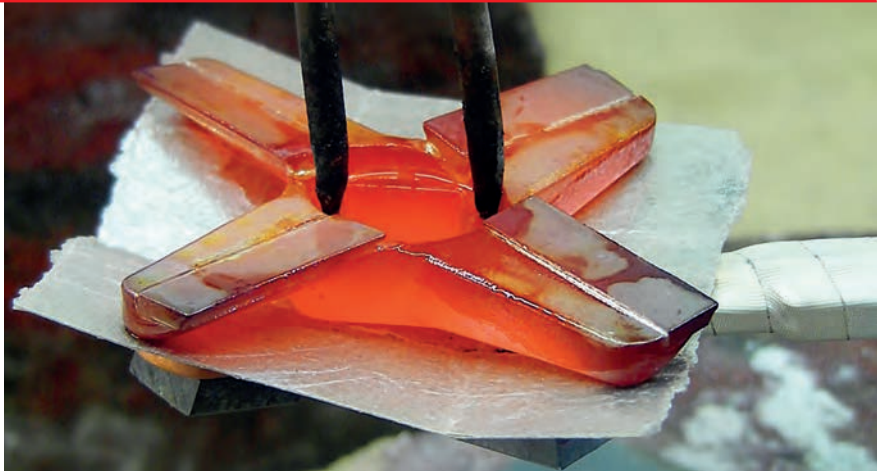
Braze-fitting carbide metal blades
