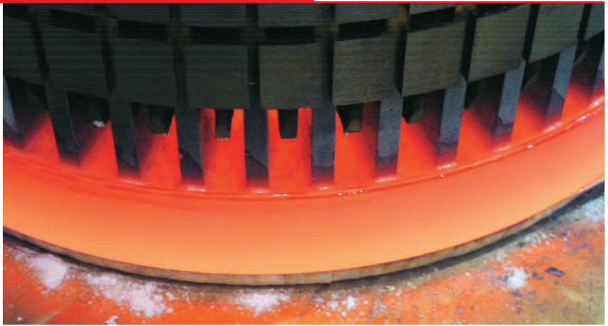
Short-circuit ring at 780°C
