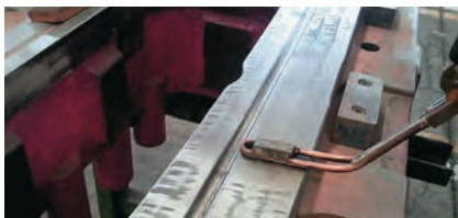
Adjusted inductor design
