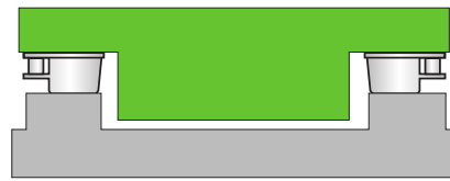
Vibration insulation concrete block or steel platform
