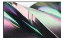
Offset chip breaker at the circumferential cutting edge
