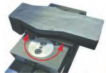
Clamping jaws with 4 pendulum supports, serrated, compensation \pm 9^\circ , pendular movable jaw, without pull-down for clamping forged parts
