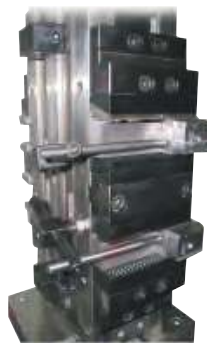
5-sided machining: Multiple clamping (blank) in RKD 125 with pull-down claw inserts
