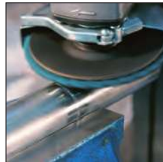
Grinding fine welding seams and removing thermal blue colouration
