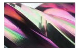
Offset chip breaker at the circumferential cutting edge
