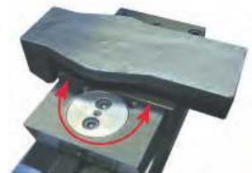
Clamping jaws with 4 pendulum supports, serrated, compensation \pm 9^\circ , pendular movable jaw, without pull-down for clamping forged parts
