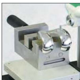
Measurement of a knee joint with the feeding device MarSurf RD 18 and the skid probe system PHTR-100
