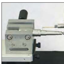
Measurement of a graduated shaft with the feeding device MarSurf SD 26 and/or MarSurf RD 18
