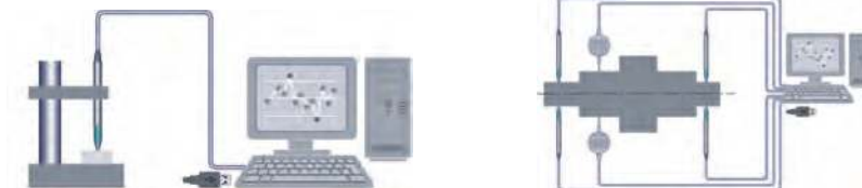
Examples when using 1 TESA USB measuring probe and multi-point measurements with multiple TESA USB measuring probes in conjunction with dial gauges.
