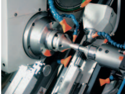
High-speed dry hobbing of planetary gears
