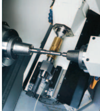
Machining area with hobbing head (direct drive)
