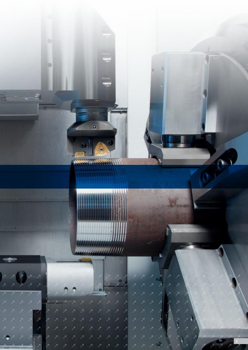
This high-precision production equipment includes two of the newest generation flat-bed turrets, each travelling on their own compound slide. Each turret features four tool stations that can be equipped with a variety of tooling systems. The change holders in the turret accommodate external and internal turning tools. The vertical design of the machine base and a generously dimensioned chip conveyor guarantee unobstructed chip flow.
