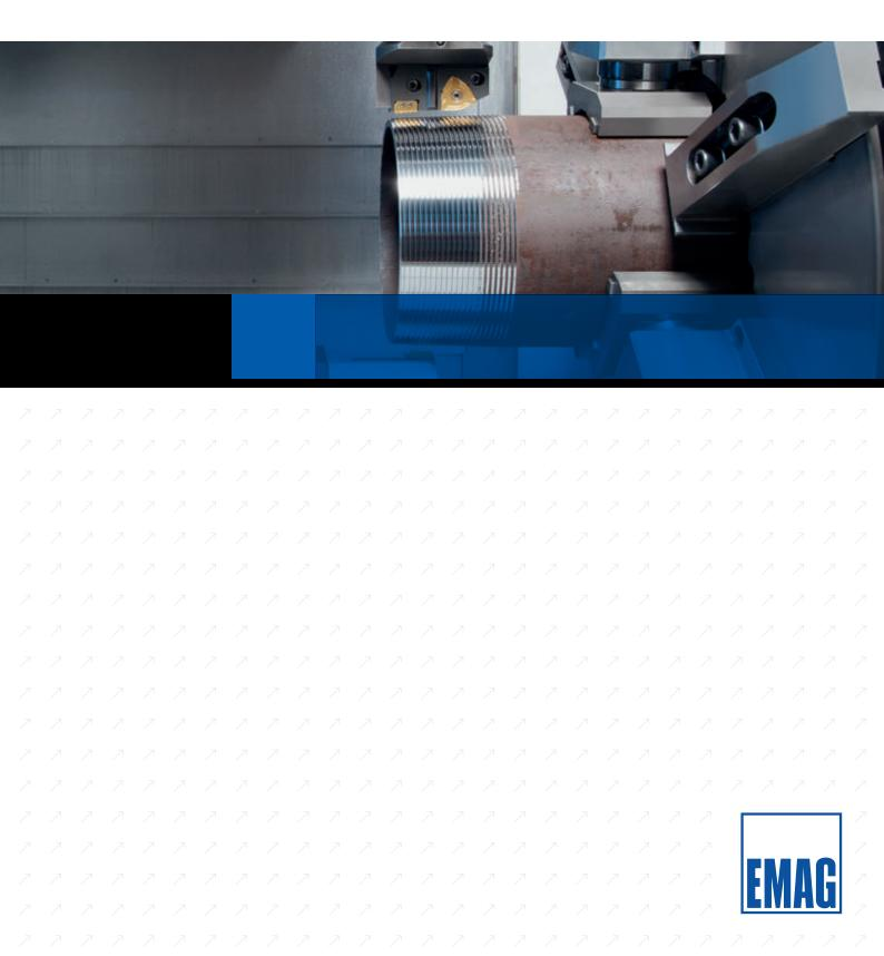
The USC 21 machine series for tube end machining and the USC 27 center drive lathe for the machining of couplings and tool joints offer customized solutions for the production of all types of thread. In fact, these state-of-the art machine tools are capable of producing all the threads on OCTG components, whether they are international (API, GOST) or a proprietary thread.
